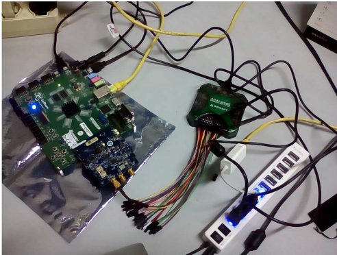
Fig. 9. Picture of the compact testbench. The ZedBoard hosts the AD9434 evaluation board. The Analog Discovery 2 signal generator is also visible.
